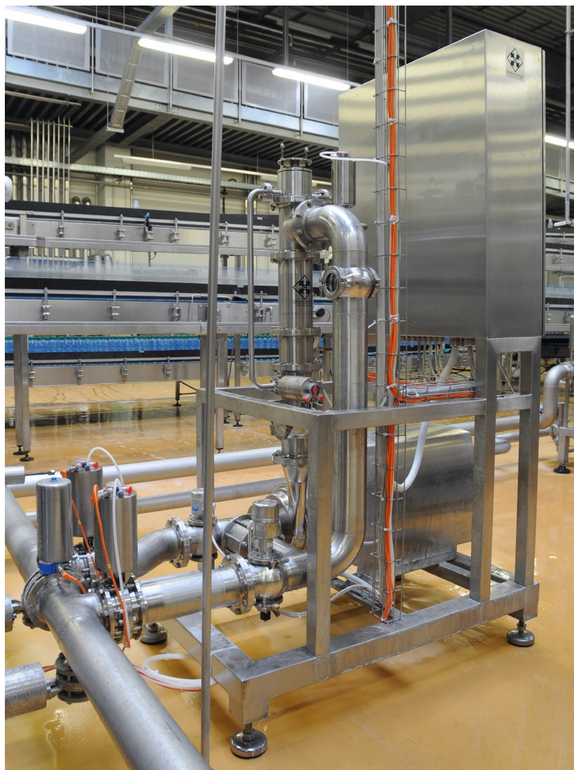
Up to 33.000 liters/h of unchilled product can be stabilised
