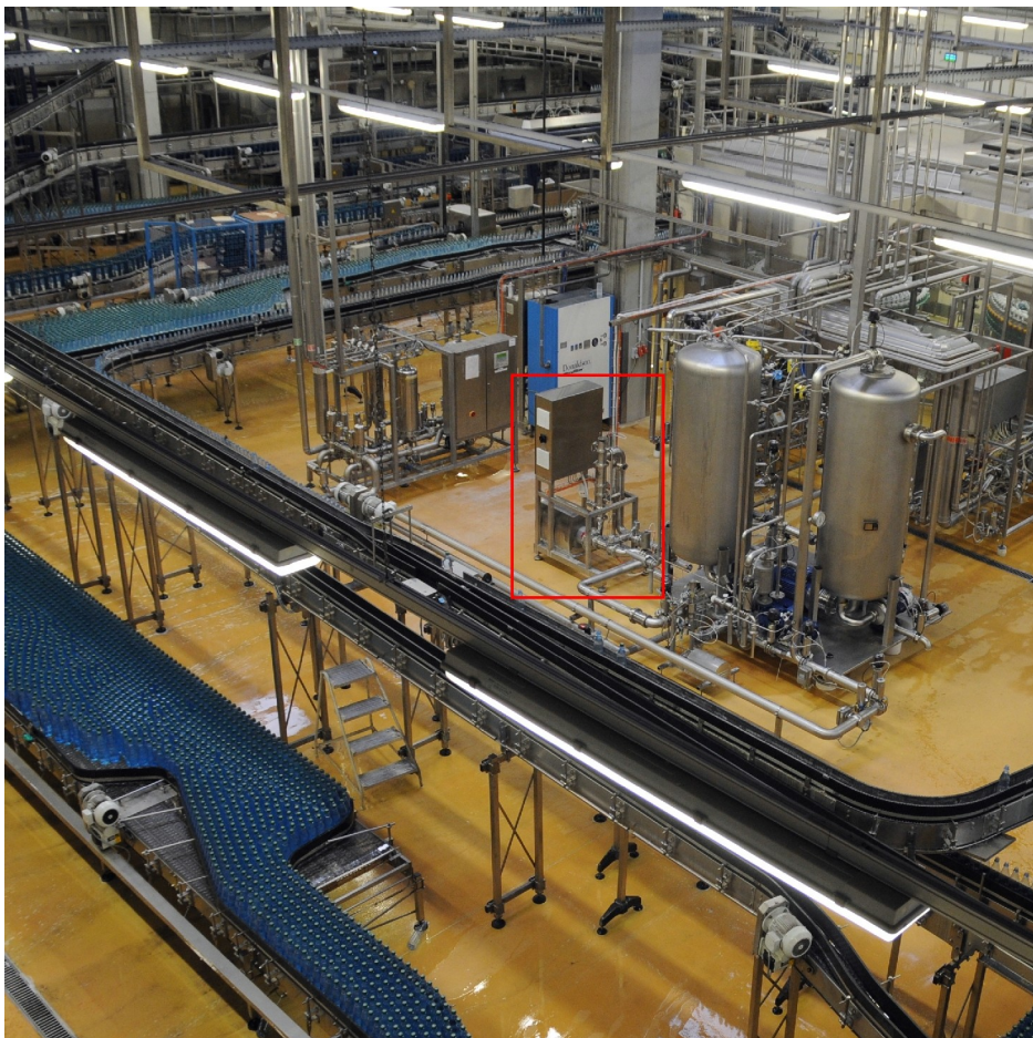
The mixing system was supplied as a plug&play version and is controlled by the respective line charger
